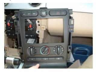
Step 8: Remove screws securing radio to the vehicle, and take the original radio out of the dash.
