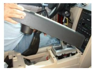
Step 4: Remove console side panels on both driver and passenger sides.
