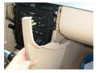
Step 5: Remove bolts securing radio bezel and AC controls.
